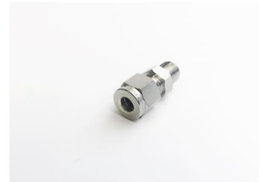
SYRINGE METRIC FITTING 1/8 NPT X 6 MM TUBE OD
